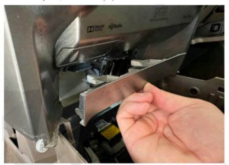
The radio will now pull straight outwards. Disconnect (2x) harnesses shown on the next page which also shows entire connection diagram.
