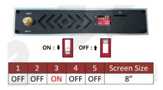
Disconnect power before adjusting dip switches.
