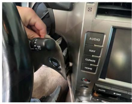
2. Remove this passenger side panel using a plastic pry tool. Remove the 10mm bolt securing screen assembly
