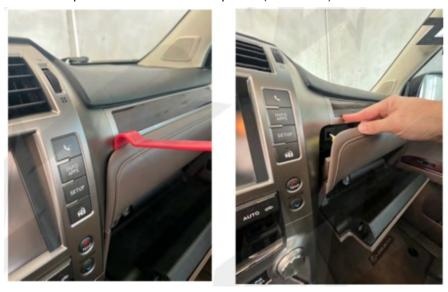
3. Remove both left and right side panels shown here. Remove 10mm bolts securing radio in sub-dash covered by these panels.
