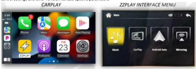
To enter the ZZPLAY Interface Menu from the CARPLAY system, locate the ZZPLAY tile and select it. If there is no phone connected, simply using the activation button (which normally brings you into CARPLAY mode) will enter you in the ZZPLAY Interface Menu.
