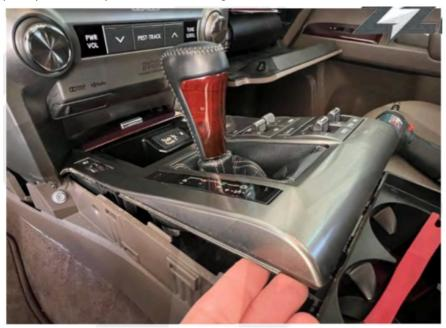
7. Disconnect (5) plugs. Two that are not shown are connected to the AUX / USB hub. NOTE: with the USB hub disconnected, 'AUX' will not display as a source choice!
