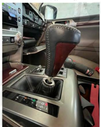
5. Remove the shifter by twisting it off.
