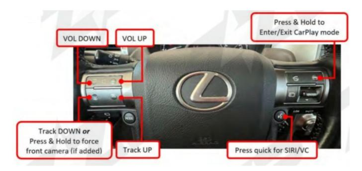
**ATTENTION:** RADIO MUST BE ON AUX MODE OR BT AUDIO (OEM) TO HEAR AUDIO FROM CARPLAY THROUGH THE SPEAKERS
