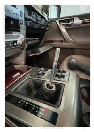
6. pull up this dash piece after removing the shifter.
