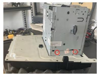
2. Carefully lift and lay down the tuner side on the back of the screen like shown. NOTE: be careful not to break ribbon cables!
