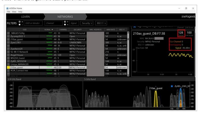
(In the example given above, we can see that Channel 128 is less used, with "0" co-channel and overlapping signals, which indicates a good environment for wireless- transmission)
