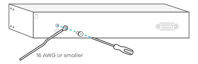
To help protect against lightning and interference functions, secure a green/yellow ground cable to the Switch.
