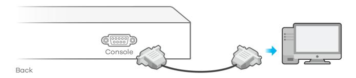
Terminal emulator configuration: VT100 terminal emulator 9600 bps or 115200 bps No parity, 8 data bits, 1 stop bit No flow control
