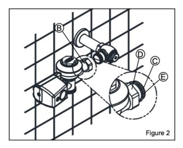
2.) Prior to inserting the flush valve tailpiece (B) into stop valve, be certain that the O-ring seal (C) is located in O-ring seal groove at the end of the tailpiece and the locking nut (D) and locking snap ring (E) are located as shown. Care should be taken not to damage the O-ring when inserting the tailpiece into the stop valve. If lubrication is needed, wetting the O-ring with water will be sufficient.
