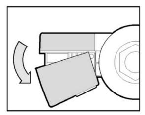
**STEP B** Pull cover off by rotating battery side forward and out.
