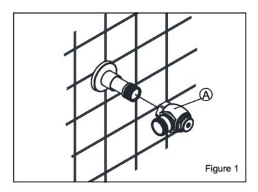
1.) Install stop valve assembly (A) using proper size supply escutcheon and sweat solder adapter kit if applicable. Thread sealing compounds should be used on male NPT threads only.
