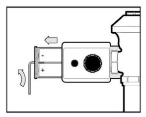
**STEP A** Use battery compartment wrench to remove battery compartment tray.
