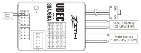
When functioning purely as an UBEC for multi-channel parallel output: The Red/Black JR connectors can be connected to relevant devices like receiver, flight control for providing (up to) 8-channel parallel voltage output & current output.
