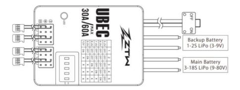
When the unit is used for connecting the gyro and servos on a helicopter.
