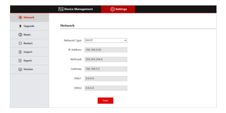
Dynamic Address(DHCP)(Default acquisition method): The joystick controller will request an IP address from the router automatically. After the request is successful, it will be displayed on the joystick controller's display. The display format is: "Local IP: 192.168.x.xxx".
