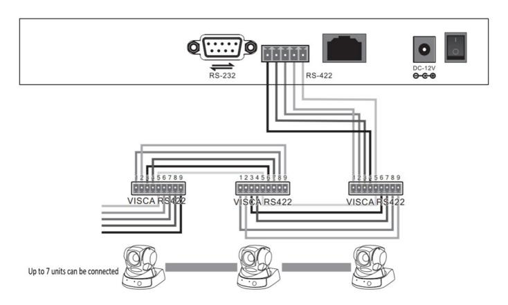
1. Using RS422 bus connection method, the third pin Ra of the joystick controller connect to TXD IN- of the camera, the fourth pin Rb of the joystick controller connect to TXD IN + of the camera, and the first pin Ta of the joystick controller connect to RXD IN- of the camera, the second pin Tb of the joystick controller connect to RXD IN- of the camera.
