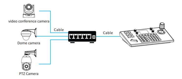
Camera and keyboard need to be connected to the same LAN.
