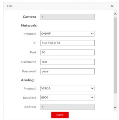
(Input the device number, corresponding IP address, port number and user name and click save.
