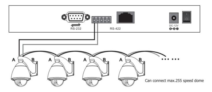
Control Output: RS485+ of PTZ camera connect to Ta of joystick controller & RS485- of PTZ Camera Connect to Tb of Joystick controller.
