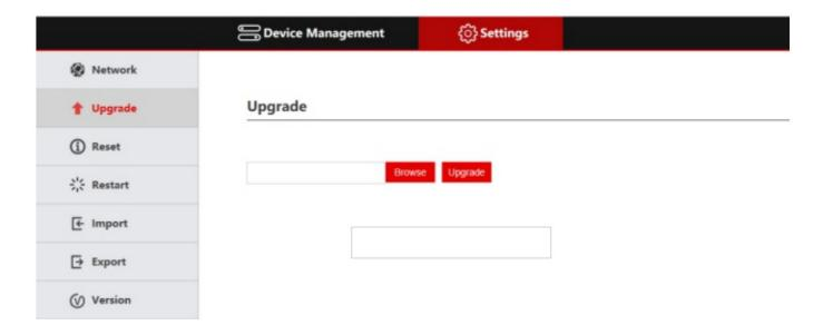
Upgrade function is used as the maintenance and update joystick function. After entering the upgrade page, select the correct upgrade file and click "Start". The device will automatically restart after the upgrade is completed.
