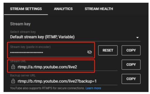
4. Copy and paste the server URL / stream key or persistent stream key into the RTMP settings of the encoder.
