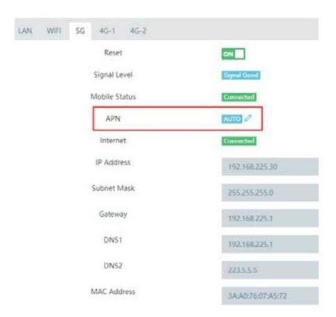
**APN setting:** After clicking the pen icon in the red mark box on the above picture, turn off "APN auto" and fill in "APN". Please ask your network operator or search online to find the APN of your 4G LTE network. When the APN setting is changed, don't forget to restart the device to take effect.
