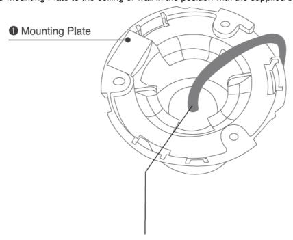
**Note:** The cable should be though the Mounting Plate.
