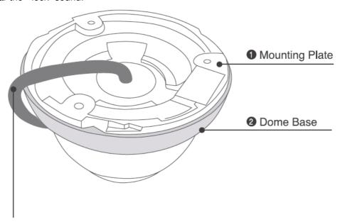
Note: The cable should be fixed on the slot hole.
