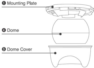
• Step 4: Install the O Mounting Plate to the ceiling or wall in the position with the supplied screws.
