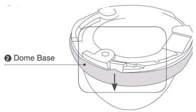
• Step 3: Remove the O Dome Cover and O Dome .
