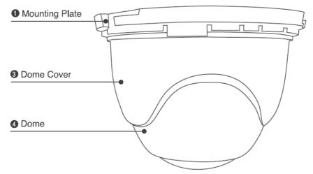
• **Step 6:** Attach the O Dome Base to the 8 Mounting Plate.then twisting Dome Base in a counterclockwise motion until hear the "lock" sound.
