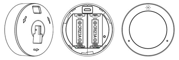
If using USB power, simply insert the micro USB cable into the USB port located over the battery slot. The LED indicator will start blinking.
