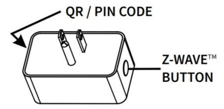
SmartStart enabled products can be added into a Z-Wave network<sup>™</sup> by scanning the Z-Wave QR Code<sup>™</sup> present on the product with a controller providing SmartStart inclusion.
