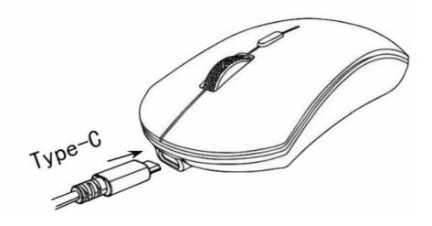
Charging cable connected to the computer is USB, charging when the red light, the charging process is about 1-2 hours, charging complete the red light goes ot
