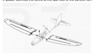
Unscrew the provided thumbscrew for the main wings. Connect the main wings, making sure both are touching the fuselage. Install the thumbscrew again to lock the main wings in position.
