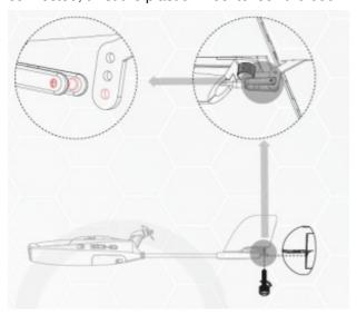
2. Install the horizontal stabilizer and make sure you're matching the hole on the tail section. Use the provided thumbscrew to lock the horizontal stabilizer in place. Connect the clevis to the last hole of the control horn
