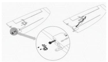
7. In case you need to change a servo: Simply remove the screws that hold the servo connectors on the wings, disconnect the old servo and connect the new one, re-routing the cable in the same way it was before. Screw the assembly back on and you're ready!
