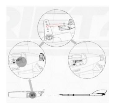
1. Install the tail boom following the graphics. The pushrod goes in the middle hole of the servo arm. Don't forget to lock the clevis against the pushrod when you're set. The tail should align perfectly with the motor. Once all is connected, twist the plastic wheel to lock the boom in position.
