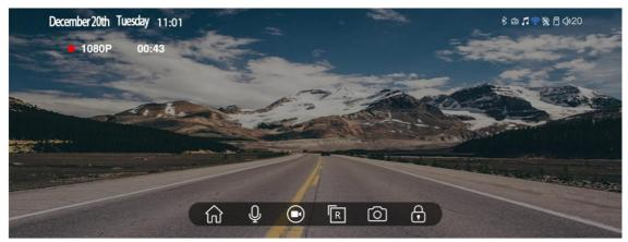
**Note:** In the video preview interface, swipe the screen left and right, you can switch the pre-recording, post-recording, double-recording lens display interface; swipe up and down the left and right areas is to adjust the camera perspective.
