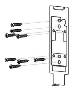
3. Attach the device to the backplate
