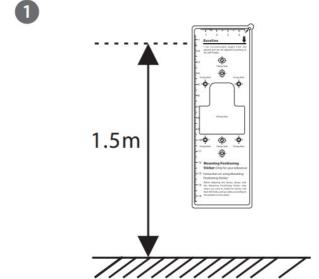
2. Fix the backplate on the wall using wall mounting screws
