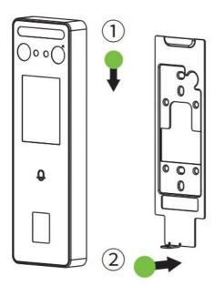
4. Fasten the device to the backplate with a security screw
