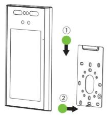
4. Use the safety screw to fasten the device to the back plate.
