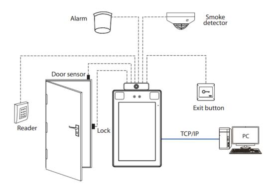
**Door Sensor, Exit Button & Alarm Connection**
