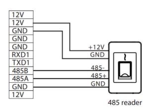
**Note:** 485A and 485B can be connected to the barrier gate or the 485 readers, but cannot be connected to the gate and the reader at the same time.
