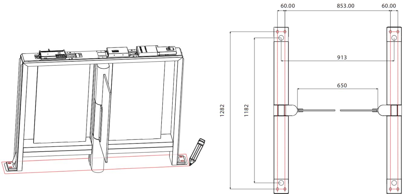
5. Take the turnstile aside and use the electric drill according to the drawn screw holes.
