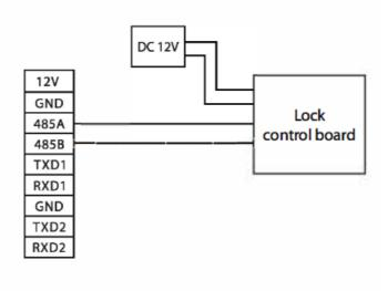
**Notice:** One lock control board could be powered by LockerPad-7B, but more than one board, they need be powered by independent power.
