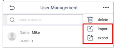
It is used for multiple devices to share a set of user data, and only supports importing and exporting user data via U disk.
