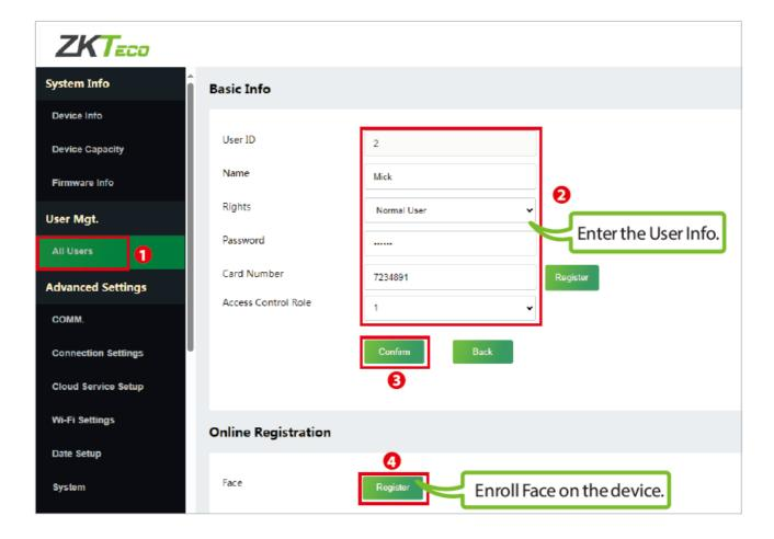
After entering the basic information of the user, click [Confirm], and then select the face and click [Register]. Follow the device prompts to face the camera and record the face until the LED indicator turns green.
