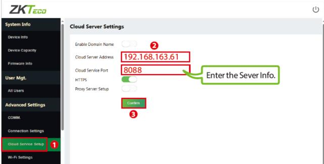
**Cloud Server Address:** This is the IP address after the software installation. Cloud Service Port: Default is 8088.
