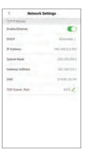
Tap Main Menu > System Settings > Network Settings, set the IP Address. The device will communicate with the PC via the Ethernet parameters. To use Cloud Server Setting set Server Address and Server port according to the server.
