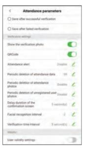
If it is enabled, the camera can recognize the QR code image on the ZKBioSecurity Mobile APP captured by the lens or the QR code scanner. Find the attendance QR code on the ZKBioSecurity Mobile App. Align it with the QR code scanner at the bottom right corner of G4[QR]. You can check in/out when verification is successful. About how to set the attendance QR code, please refer to Chapter 7.5 of the [ZKBioSecurity Mobile APP User Manual].
