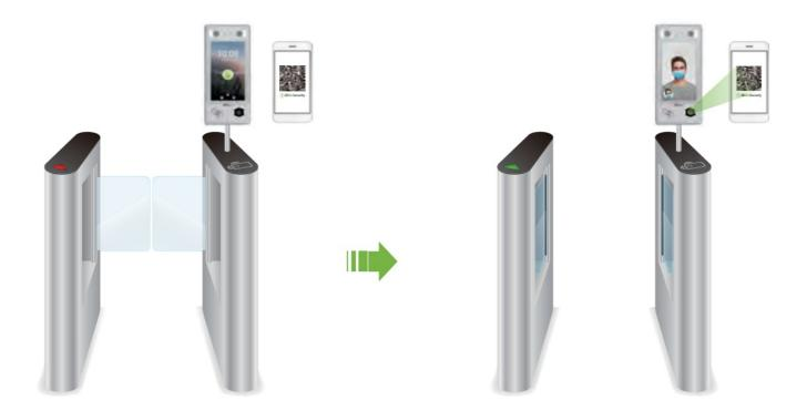
Find the access control QR code on the ZKBioSecurity Mobile App. Align it with the QR code scanner at the bottom right corner of G4[QR]. The gate will open when verification is successful. About how to set the access control QR code, please refer to Chapter 7.5 of the [ZKBioSecurity Mobile APP User Manual].
