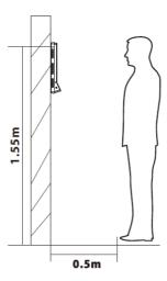
For the user's height ranging from 1.5m to 1.8m, the recommended device height is 1.55m from the ground. It can be adjusted and installed according to the user's average height.
