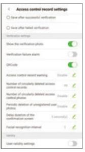
If it is enabled, the camera can recognize the QR code image on the ZKBioSecurity Mobile APP captured by the lens or the QR code scanner.
