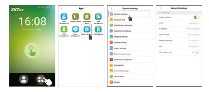
**Tap Main Menu** > System Settings > Network Settings set the IP Address. The device will communicate with the PC via the Ethernet parameters. To use Cloud Server Setting set Server Address and Server port according to the server.
