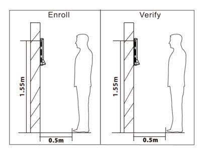
The registration and verification position of the device shouldn't be changed to avoid affecting the verification accuracy. If it is necessary to move the device, then move it horizontally keeping the vertical height the same.
