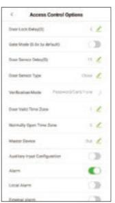
**Tap Main Menu** > Access Control > Access Control Options to enter the Access Control Options setting interface and set relevant parameters of the access control.
