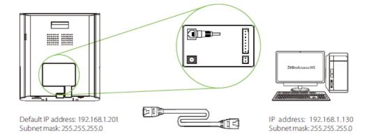
Click on [COMM.] > [Ethernet] > [IP Address], input the IP address and click on [OK]. **Note**: In LAN, the IP addresses of the server (PC) and the device must be in the same network segment when connecting to the ZKBioAccess IVS software.
