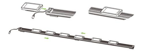
Step 3: Reinstall the clips on the guideway.
