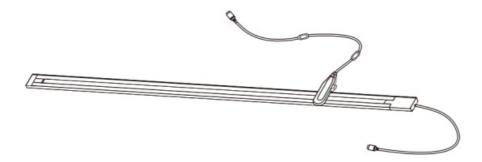
**Step 5:** Secure the power connection cable to the magnetic conductive strip by rotating it 90° counterclockwise as shown in the figure below. This method supports the installation of multiple power connection cables.
