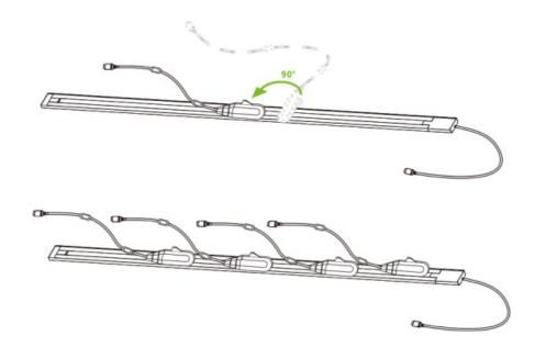
**Step 6:** First, connect the guideway to the magnetic conductive strip, and then turn on the power to the magnetic conductive strip. Once the guideway is powered up, the device receives energy from Wireless Metal Contacts. This wireless charging technology is similar to the Qi method used in cell phones, ensuring safety and harmless.
