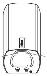
Fig. 5 Removing the protective cover
