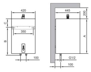
Fig. 3 Vertical installation on a wall
