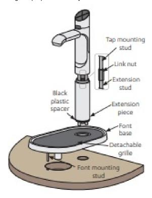
Secure Font & Tap, attach drain (underneath)
