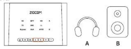
Press the A/B button to enter pairing mode, the white LED will flash, the transmitter will automatically pair the Bluetooth device.
