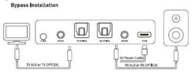
Use the BYPASS function if your TV only has ONE OPTICAL Output which is currently occupied by your AV receiver or sound bar Toggle between BYPASS and Bluetooth mode using a simple switch. No need to unplug cable. In Bypass mode, -8T5809" can be used as a decoder to convert audio between 3.5mm AUX and optical output
