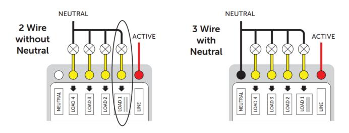
Always use a Neutral wire where possible. When operating without a neutral connection, a small amount of power is used via LOAD 1 when switched off. This may in some instances result in lights not completely turning off. Dimmable loads might be fixed by increasing to at least 2 lights with a load >10W. Non-Dimmable loads may require a bypass/load correction device fitted if the load is insufficient.
