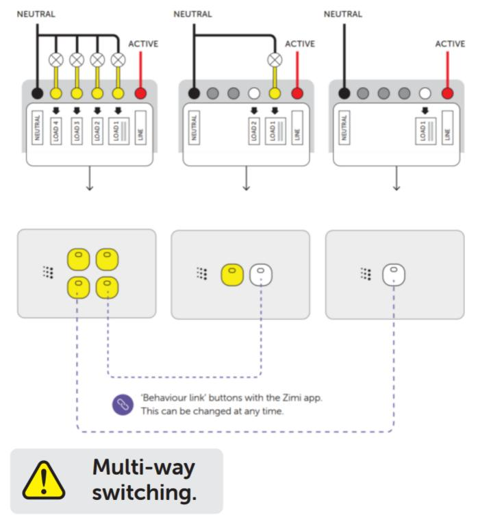
The Powermesh Multi Purpose Switch SHOULD NOT be wired with any other type of switches.
