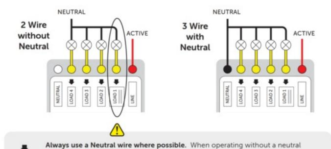
connected, a small amount of power is used via LOAD 1 when switched off. This may in some instances result with lights not completely turning off. **Dimmable** loads might be fixed by increasing to at least 2 lights with a load >10W. **Non-Dimmable** loads may require a bypass/load correction device fitted if the load is insufficient.
