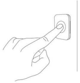
• The Smart Button is water-proof and thus suited for indoor and outdoor use. For use as a doorbell mount the button outside the door with the double adhesive tape.
