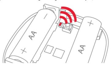
6. When the LED stops flashing, the Smart Humidity Sensor has successfully joined the Zigbee network.
