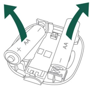
2. Replace the batteries respecting the polarities.
