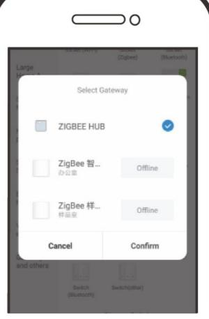
Make sure your smart phone and ZigBee switch module are under the same WiFi network at 2.4 GHz connection. Confirm when the beep sounds continuously rapidly (twice a second).
