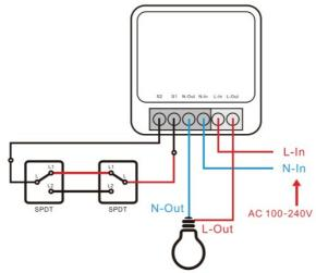
⚠ S1/S2 can connect with the rocker light switch, or it doesn't connect. To ensure safety, do not connect the neutral wire and live wire to it.
