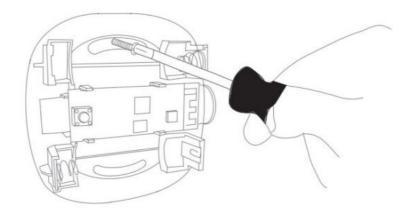
3. Insert batteries respecting the polarities.
