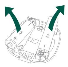
2. Replace the batteries respecting the polarities.
