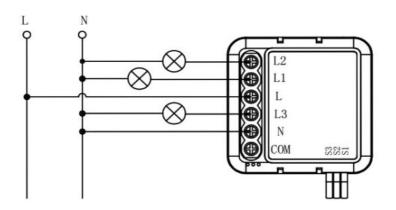
3CH Zigbee Switch Module Without Switch
