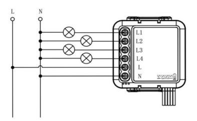
4CH Zigbee Switch Module Without Switch
