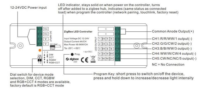
1. Under RGBW mode, W channel can only be turned on through color temperature control command (RGBW will be identified as RGB+CCT by zigbee). Color temperature control will mix RGB channels as 1 channel white and then make color tuning with the 4th channel white. Once turned on, the brightness of white channel will be controlled together with RGB channels.
