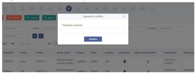
**Note:** The detection cycle is related to the battery life. The more frequent the detection cycle, the faster the battery consumption and the shorter the service life.
