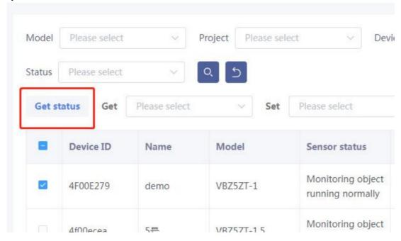
2 The query delay is related to the ZETA protocol. If it is in real-time downlink mode, it can be inquired in real-time. If it is in ACK downlink mode, it needs to wait for the uplink cycle.
