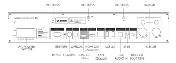
**Antenna Installation Instruction:** Please install the three antennas from the accessories onto the antenna interfaces shown in the image above.
