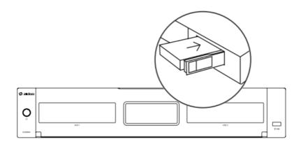
**Note:** Do not load or replace the hard disk while the device is powered on to avoid damage to the device or hard disk data. Brand new hard disks need to be formatted before loading. This device supports the following hard drive formats: EXT3, EXT4, NTFS, FAT32, EXFAT.
