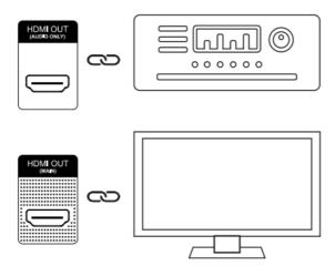
**Note:** The dual-port output mode is suitable for AV receivers that do not support resolutions higher than 4K or 3D functionality, and when the display device supports resolutions higher than 4K or 3D functionality.
