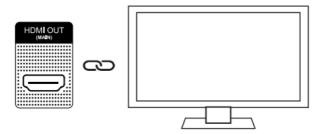
3. HDMI Dual-port Output (audio and video separate output): With both the TV and media player powered off, insert one end of an HDMI cable into the HDMI OUT AUDIO ONLY port of this device and connect the other end to the AV receiver. Then, use another HDMI cable to connect one end to the HDMI OUT MAIN port of this device and the other end to the TV's HDMI IN port. This connection will enable the separation of audio and video output.
