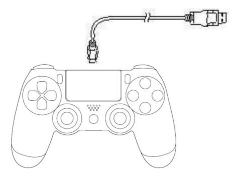
To a USB port on the P4 console system. USB cable (supplied with the P4 console system)
