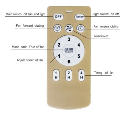
Match coda: After hear the "beep' sound when tum on the power, at the same time passcode match/Trun off fan" button for 3 seconds. When remote control sound twice "beep" then the code has matched If code doesn't match successfully, please shut off the power and wait for about 1 minute, then repeat the last action
