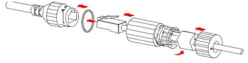
CAUTION! You need to mount the rubber ring onto the network cable interface first.
