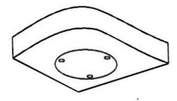
3. Fix the adapter plate to the ceiling.
