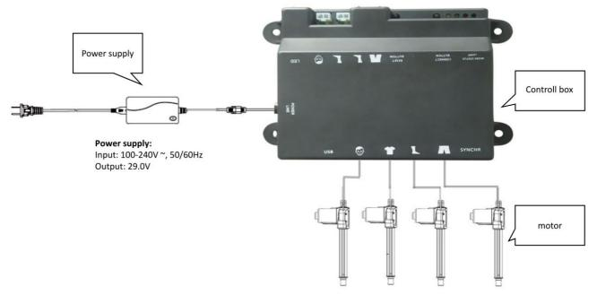
**Motor:** By pairing the remote control with the control box, the motor can be controlled up and down.
