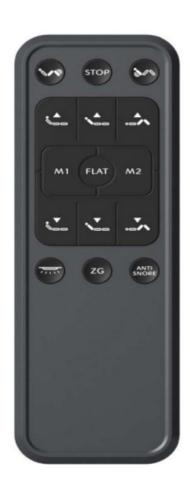
Press button and not release, the actuator M1 move up, release the button, the actuator stop moving;
