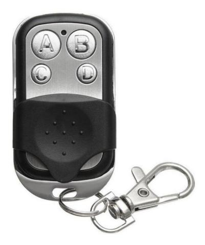
Total have 24 coding BYTE0+BYTE1+BYTE2+end bit Total have 24 coding, BYTE0+BYTE1+BYTE2+end bit also can set as rolling code, the address code of per controller are all different rolling code can achieve one to one function, means one remote control can only control one receiving equipment. BYTE2 is the key code value, the code value of per key are fixed.0 03 Below is the picture, show key value of K1=01, the address code is 20,03
