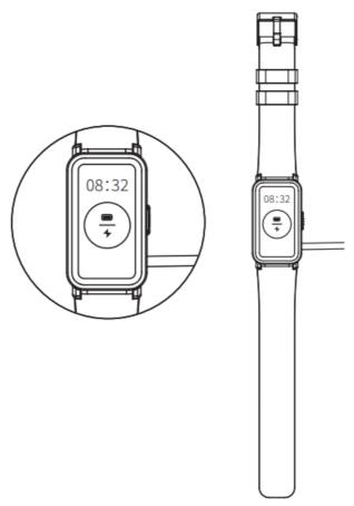
To check the charging progress, press the button on the side. A solid battery icon indicates a full charge.
