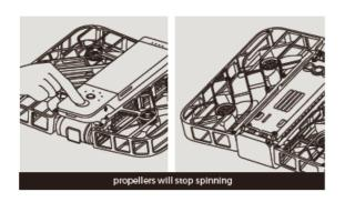
At the end of the flight or during continuous flight modes, place your hand 20cm below the device and it will automatically land in your hand and the propellers will stop spinning
