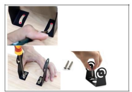
2. Then install the bracket with supplied screws, keeping them loose for adjustment.
