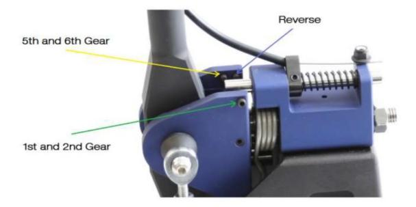
Using the gear lever, shift the gearbox into 1st and 2nd. You may need to screw the (green arrow) grub screw out to achieve this.
