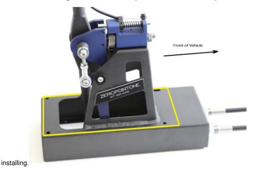
The yellow line shown on the base of the ZPO shifter is a guideline of where the foam/sealant should be placed. Insert the shifter from the bottom of the vehicle into the tunnel allowing the 4 base bolts to line up with the holes in the tunnel. Then from inside the vehicle fasten with the 4 nuts provided. Do not put the base plate onto the base until the nuts are fully tightened, you may need to use a hex/torx tool to hold the 4 bolts while nuts are tightened up.
