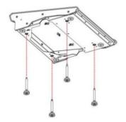
When using ZerOS Wings behind FLX, feet are available which raise ZerOS Wing to match the rear of the console. These are available in packs of four (order code 0021- 000006-00). These feet simply screw into the bottom of ZerOS Wing, as shown.
